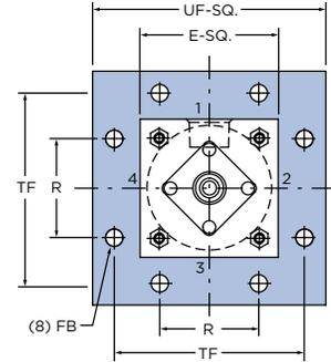
**MODEL CJ (BLIND HEAD SQUARE MOUNT) 14" THROUGH 20" DIAMETER BORE**
