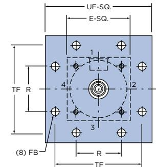
**MODEL DG (ROD HEAD SQUARE MOUNT) 14" THROUGH 20" DIAMETER BORE**
