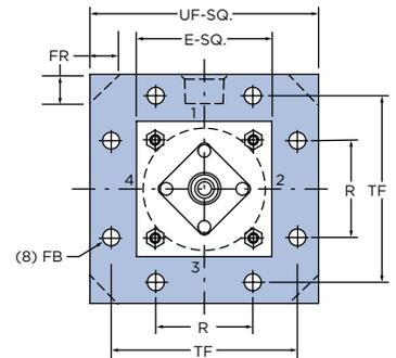
**MODEL DD (ROD END FLANGE MOUNT) 10" THROUGH 12" DIAMETER BORE**
