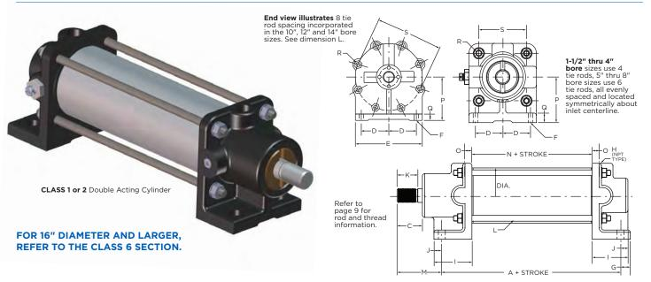
Model "A" is used primarily in applications requiring straight-line push-pull motion where cylinder can be mounted on a flat surface. Intermediate supports can be furnished in cases where ratio of cylinder stroke to bore is large, to prevent excessive deflection and resulting wear on cups and packings.
