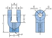
**Clevises** of high grade malleable iron are available for all standard model and size Class 1 and 2 cylinders. Clevises for any diameter cylinder are threaded for that particular standard 1 rod end. Class 1 and 2 cylinders with oversize rod and Class M cylinders will therefore require a larger clevis unless the rod end is turned down. Be sure to specify when ordering. Special clevises available made to order.
