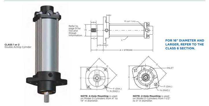
Model D is similar in construction to Model C, except that the piston rod is extended through the mounting base. It may be mounted on any flat surface in which an opening can be provided for the protruding cushion boss and extension of the rod. It is used extensively in applications of inward pulling power.
