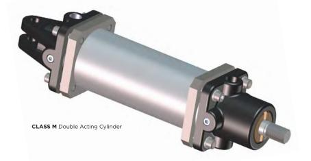
NOPAK Class M cylinders are strong and rugged in construction, especially designed for heavy duty applications in mines, quarries, steel mills, and in the heavy construction industries. Maximum system pressure is 650 PSI in all diameters to 4" – and 450 PSI in diameters of 5" and larger. The Class M construction is available in a full range of sizes and models (mountings) up through 14" in diameter for air, water or oil hydraulic service.
