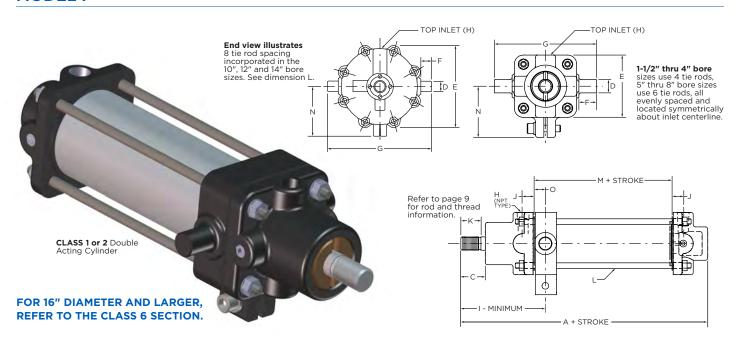
The Model F Trunnion Mounting provides smooth, dependable cylinder power where oscillating movement is necessary in connection with heavy side thrust. Trunnion location is indicated by dimension "I," which is minimum and furnished as shown unless otherwise specified; it may be increased within limits of cylinder tubing length.
