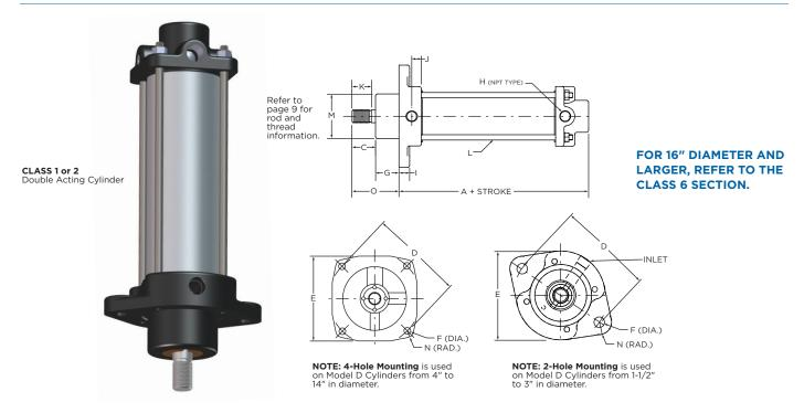
Model D is similar in construction to Model C, except that the piston rod is extended through the mounting base. It may be mounted on any flat surface in which an opening can be provided for the protruding cushion boss and extension of the rod. It is used extensively in applications of inward pulling power.
