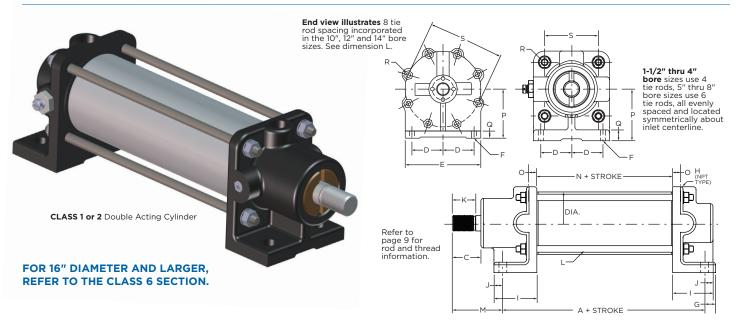
Model "A" is used primarily in applications requiring straight-line push-pull motion where cylinder can be mounted on a flat surface. Intermediate supports can be furnished in cases where ratio of cylinder stroke to bore is large, to prevent excessive deflection and resulting wear on cups and packings.
