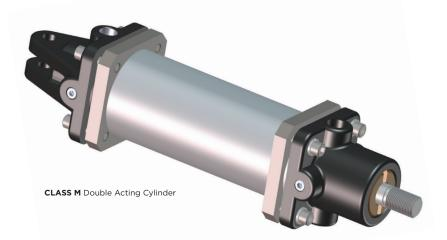
NOPAK Class M cylinders are strong and rugged in construction, especially designed for heavy duty applications in mines, quarries, steel mills, and in the heavy construction industries. Maximum system pressure is 650 PSI in all diameters to 4" – and 450 PSI in diameters of 5" and larger. The Class M construction is available in a full range of sizes and models (mountings) up through 14" in diameter for air, water or oil hydraulic service.
